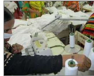
Photo of non-conformity Eye guard found displaced.JPG
