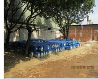
Photo of non-conformity Chemicals were not stored properly.JPG
